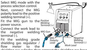
shielding gas cylinder, then connect the shielding gas hose from the rear of the power source to the regulator / flowmeter outlet.
