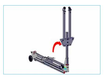
4. While in this vertical position remove ball lock pin from its stow hole.
