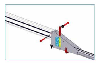
28. Move leg assembly to required position.
