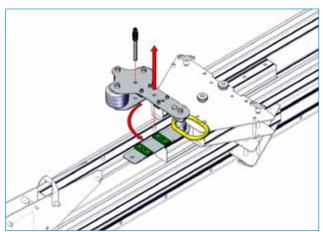
For trolleys stowed on underside upright, if stow pins available, removal can only take place when the upper A-frame assembly is rotated out of the way, or when gantry is set up.
