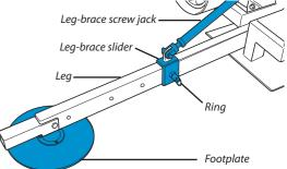
Pull the ring to unlock the leg-brace slider and lower the leg from vertical into horizontal position.
