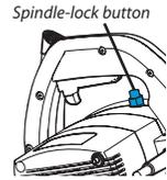
Before installing a new blade, **check that both blade flange discs are clean**. Place a new or **sharpened blade on the back flange disc**, so that the marked side of the blade is facing outwards and the arrows on the blade are facing in the same direction as the rotation direction markings on the inside of the blade case.
