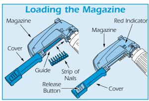
hear a click as the fastener guide slides back and arms the firing mechanism.
