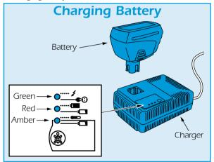
The green lamp illuminates to confirm that the charger is connected to a live power supply.
