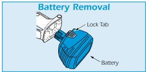
**Fit the battery to the Drywall Screwdriver**, simply push into the base of the handle until it clicks into position.
