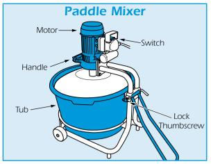
When the mix is ready to use switch the unit OFF, unlock the thumbscrew and raise the motor using the handle. It may be necessary to align the paddles square on to the base frame to ensure the paddles do not foul the tub.
