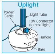
Take the Uplight to the work area and site it so that it is away from pedestrian traffic but near enough to the work to provide sufficient light.
