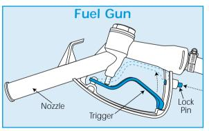
To transfer diesel begin by removing the gun from its holster, place the nozzle into the container being filled and lock the trigger open.
