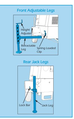
**Stand the unit on a firm, level surface** strong enough to bear its weight. DO NOT use on slopes, soft ground or where there is a risk of subsidence.
