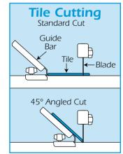
Set the guide bar to the correct width of cut required, this distance should be for the piece required and not for the waste piece.
