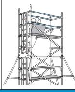
When building beyond a 3.2 m platform height Tower Continue to add Span and Ladder Frames, Diagonal Braces and Trapdoor Platforms as shown in the previous steps Always add Horizontal Guardrails from the protected position within the Trando
