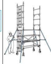
Fit 4 Diagonal Braces (Blue) in opposing directions between the 3rd and 5th Rungs and the 5th and 7th Rungs
