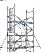
Climb the Ladder and from the protected position of the Trapdoor, fit Guardrails to the 7th and 8th Rungs (in that order), on both sides of the
