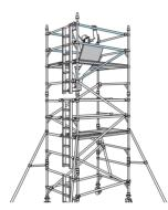
When building beyond a 4.2 m platform height Tower Continue to add Span and Ladder Frames, Diagonal Braces and Trapdoor Platforms as shown in the previous steps.
