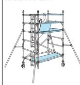
Fit the next pair of Diagonal Braces in opposing directions between the 3rd and 5th Rungs
