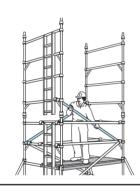
If finishing at this height (4.2 m Platform), the Fixed Deck should first be repositioned to the 8th Rung of the Tower. Fit a Trapdoor alongside it, with the Trapdoor next to the
