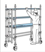
Fit 2 Diagonal Braces (Blue) in opposing directions between the 1st and 3rd Rungs. Fit an additional Ladder Frame and
