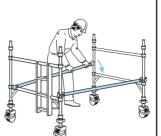
Fit an additional Ladder Frame and Span Frame Ensure the Interlock Clips are engaged.
