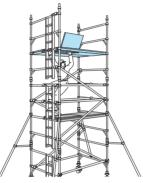
Climb the Ladder and, from a protected Trapdoor position, fix Guardrails on the 9th and 10th Rungs, in that order, on both sides of the Tower. Add a Diagonal Brace between the 7th and 9th Rung.
