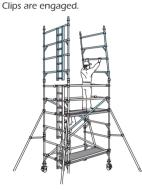
Fit the next pair of Diagonal Braces between the 5th and 7th Rungs
