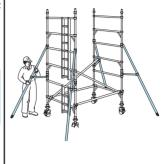
Fit a Fixed Deck on the lowest rung. Fit a Trapdoor Deck on the 4th Rung (2.0 m) with the Trapdoor next to the Ladder.
