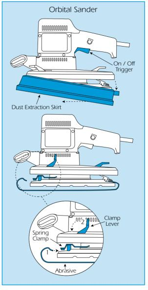
If using an Orbital or Palm Sander. With the machine switched OFF and isolated from the power supply, turn the sander on its back.
