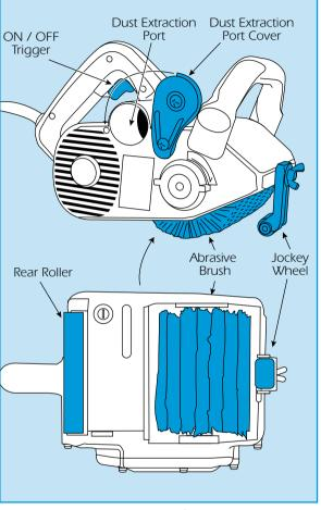
Always use the correct abrasive for the job and (where applicable) change it as soon as it becomes clogged or damaged. Never use the sander without an abrasive fitted.
