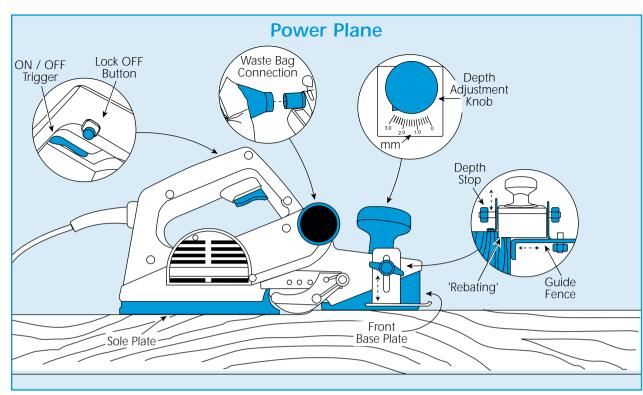
To switch the planer ON, push the lock OFF button in with your thumb, then squeeze the ON/OFF trigger.
