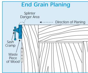
When planing across an end grain (base of a door for example) clamp a piece of waste material against the end with a sash cramp or similar to avoid splintering (see diagram).
