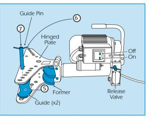
7. Push in the quide pins through the holes in the hinged-plate, the guides and the baseplate to secure, and if necessary, correct the position of the auides.
