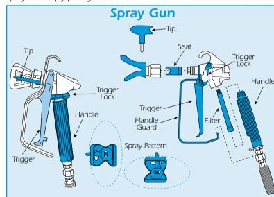
**Ensure the tip is suitable for the material you wish to spray** and the guns filter is the correct grade, (see table). If in doubt, contact your local HSS Hire Shop for advice.
