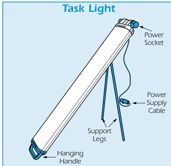
Uncoil the light's power supply cable, coiling excess lead neatly but loosely, close to the power supply and away from the work area where people can't trip over it.
