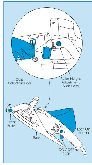
NOTE: The maximum stock removal should not exceed 2.5mm.
