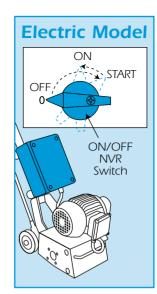
The switch is operated in three stages, OFF, ON and Start. To switch the motor ON move the switch dial clockwise to the ON position then through to the Start position, Return the dial to the ON position to start work. To switch the motor OFF simply turn the dial to the OFF position.
