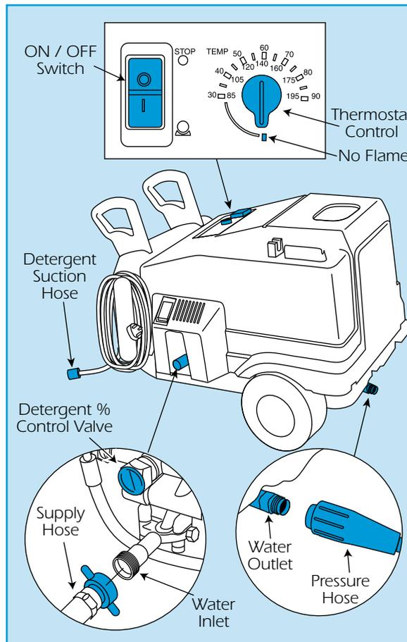
Always switch OFF the equipment when not in use. The burners exhaust get very hot so keep your distance. Never look directly into the exhaust port nor cover it at any time.
