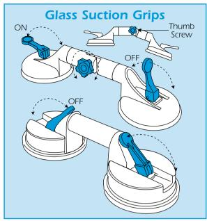
Firmly press the cup faces against the glass surface, then fully push the suction levers down, one at a time, to create the vacuum grip.
