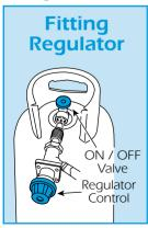
Screw the gas regulator onto the propane cylinder's valve, turning it anti-clockwise to tighten (it has a reverse thread) and tighten up with the spanner provided, then open the cylinder valve and check for leaks.
