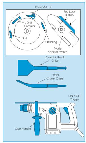
To change the angle of the chisel press the red lock button and move the selector lever to the 'chisel adjust' icon. The chisel is now free to rotate to the required angle. To lock the position and set the machine ready to work, turn the selector to the 'chiselling' icon.
