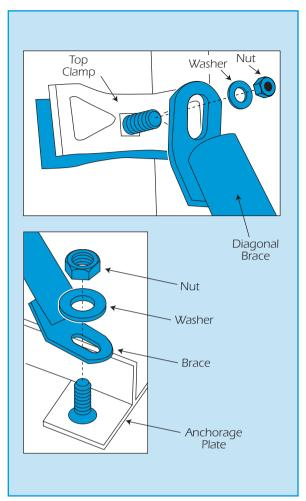
**Alternatively, anchor directly into the ground** surface using the correct type of anchor fixing.
