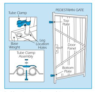
Position the next base weight at the correct distance for the pedestrian gate, then lift the door in to position.
