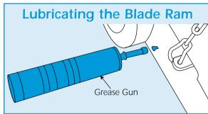
After using either model to remove 500 square metres, (long term hire only) use the grease gun provided to lubricate the blade rams.
