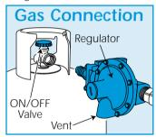
You can now connect the gas supply. To do this screw the gas regulator onto the propane cylinders valve, turning it anti-clockwise to tighten (it has a reverse thread) and tighten up with the spanner provided.
