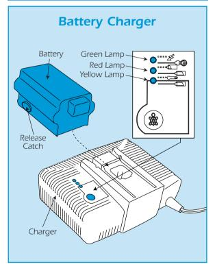
The battery charger is designed to plug straight into a standard 240V 13A power socket.
