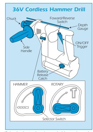
If the depth stop is to be used, this may be set by twisting the side handle to loosen/tighten the depth rod's guide.
