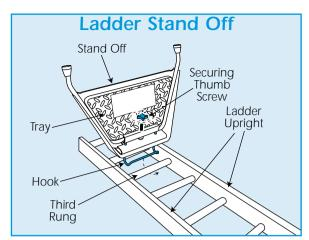
Make sure the stand off is correctly positioned against the ladder uprights.
