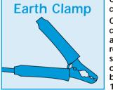
Connect the earth lead clamp to the work.
