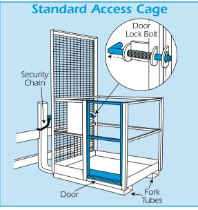
Now **lift the safety rail assembly** in the same way as the mesh panels **and engage in its slots**. All that remains is to **swing the 4 side bars out and engage their lock pins in the holes at the side of the mesh panel**.
