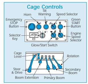
When fully lowered the unit can be driven at up to 2.1 miles per hour, when raised the speed is reduced to a maximum of 1 miles per hour.
