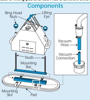
HSS offer a 200Kg and a 400Kg pad. If you need to change the pad size fitted to the unit, firstly ensure the unit is switched OFF.
