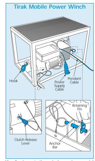
Visually inspect the winch, paying special attention to the condition of the cable and hooks. The cable should be clean and free from dust, dirt, moisture and grease. If the cable is gouged, twisted or has distorted in any way DO NOT USE IT, return it to your local HSS Lift & Shift Depot.
