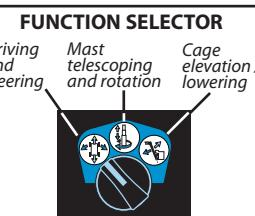
All driving speeds are authorized when the machine is stowed (machine in lowered position). When the cage or mast are raised the unit will move at a reduced speed.
