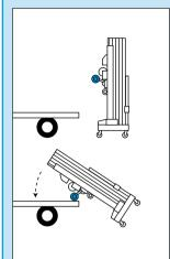
This unit can be loaded onto a flat bed vehicle with the minimum of effort.
