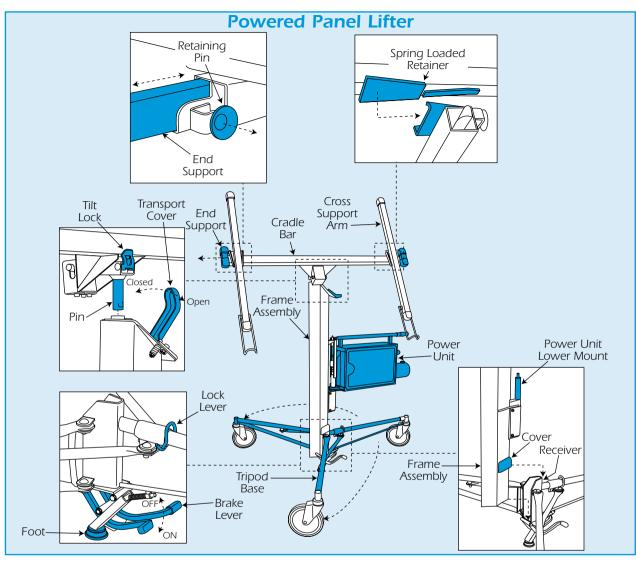
To recharge the battery, disconnect the batteries block connector and remove it from the power unit.
