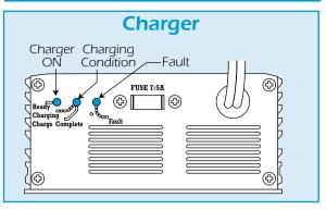
The HSS Powered Panel Lifter is powered by a 12V battery. The battery charger is supplied as a separate unit. The battery charger is designed to run from a 110V power supply via a generator, or be powered from the mains via a suitable 110V transformer.
