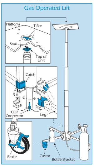
Next, **fit the platform to the top of the unit.** Lower the centre of the platform on to the top stud and tighten down by turning the T bar clockwise.
