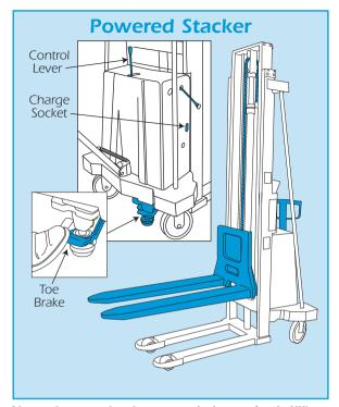
Never leave a load unattended or raised. When not in use, park the Powered Stacker on level ground where the forks will not cause a trip hazard.
