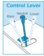
The Powered Stacker is controlled by a single lever, which has three positions (see illustration). To raise the forks, move
