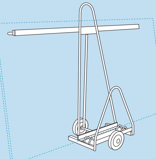
Place the load with the longest edge horizontal to the trolley, positioned centrally and with its bottom edge close to the base of the support bar. If possible, secure the load with suitable strapping.
