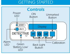
Switch the unit ON by pressing the ON button. The alarm will sound and the red 'alarm' LED will flash for approximately 5 seconds.
