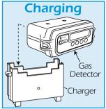
To charge the battery, simply insert the unit into the charger (see illustration), ensuring the unit is the correct way up.
