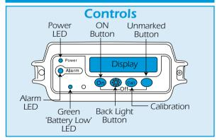
**Switch the unit ON by pressing the ON button.** The alarm will sound and the red 'alarm' LED will flash momentarily.
