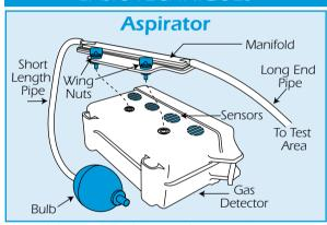
The unit is supplied with an aspirator, used to test an area prior to entry.
