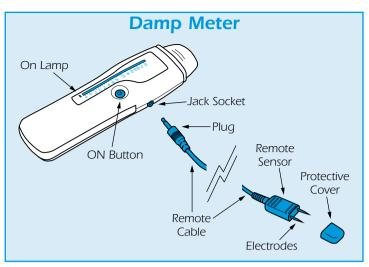
You can now reveal the twin electrodes by carefully removing the protective cover.
