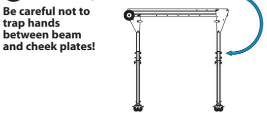
**If space is further limited for set up then the legs can be removed.**
